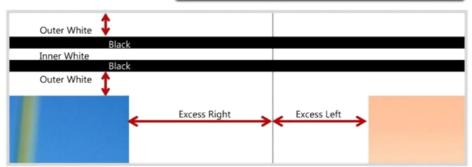
Use values **Excess Left** and **Excess Right** according to the figure above to configure an automatic left and right margin to the image in order to consider the position of the knifes cutting vertically (in the direction of media movement).
